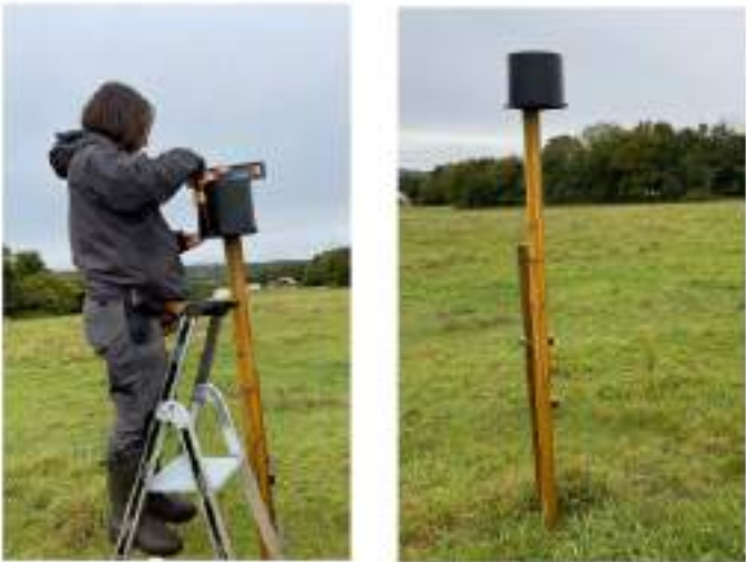
Fig. 2.23 Maintenance and deployment of a rain gauge.
