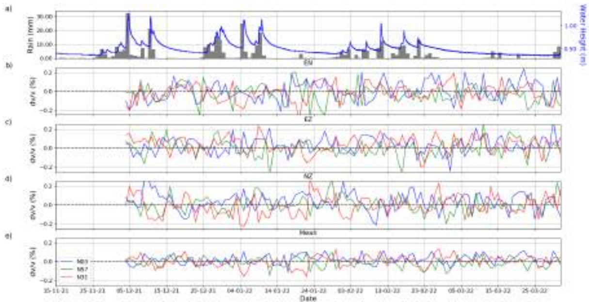
Fig. 4.18 Five-days stacked dv/v measured under 3 nodes located on limestone [8-10 Hz]. a) Daily rainfall (bars) and underground river water height (blue line) during the studied period. dv at nodes N3, N21, N57 for b) EN, c) EZ, d) NZ cross-components and e) the mean of the 3 cross-components.
