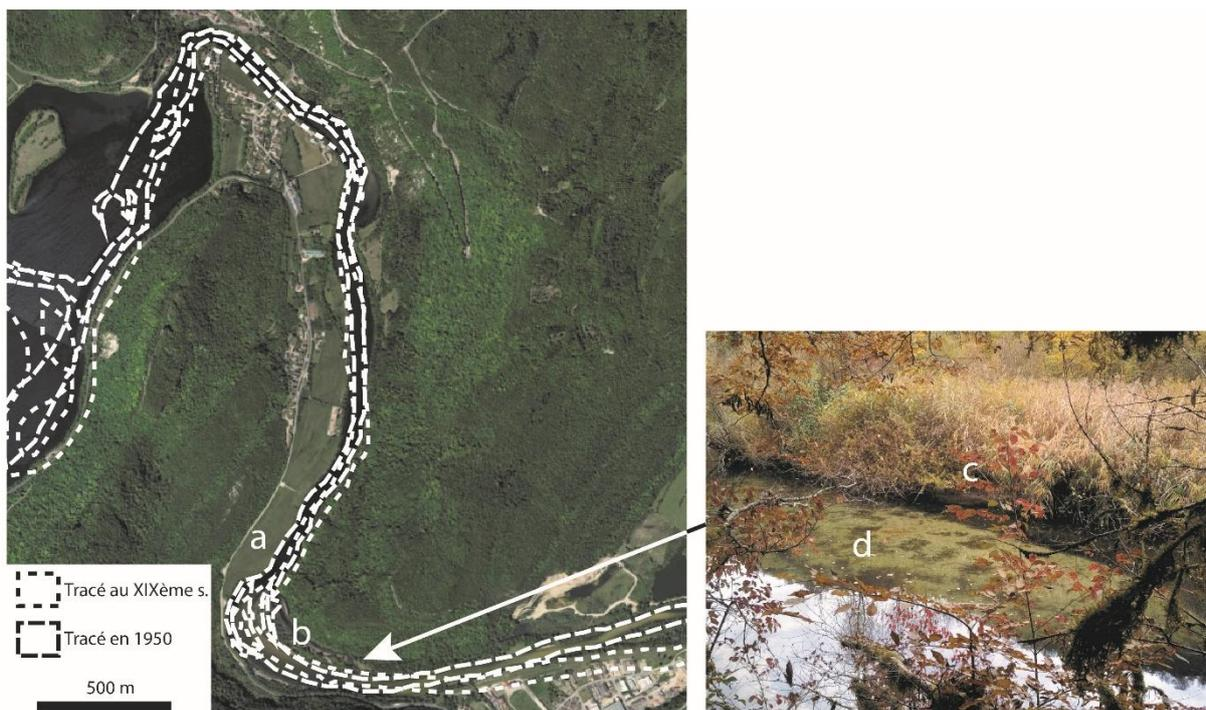
FIG. 9 : EVOLUTION DU TRACÉ DE LA BIENNE DANS LE TRONÇON DORTAN-CHANCIA. LA PHOTOGRAPHIE AERIEENNE DATE DE 2017. A : PLAINE D'INONDATION FOSSILISEE, B : ANNEXE FLUVIATILE RESULTANT DU CONTROLE DE LA LIGNE D'EAU PAR LE BARRAGE DE COISELET, C : PHRAGMITAIE JOUANT LE ROLE DE PIEGES A SEDIMENTS FINS PROPICES A L'ENREGISTREMENT A LONG TERME DES POLLUTIONS SEDIMENTAIRES, D : REMPLISSAGE SEDIMENTAIRE IRRÉGULIER DANS L'ANNEXE FLUVIATILE
