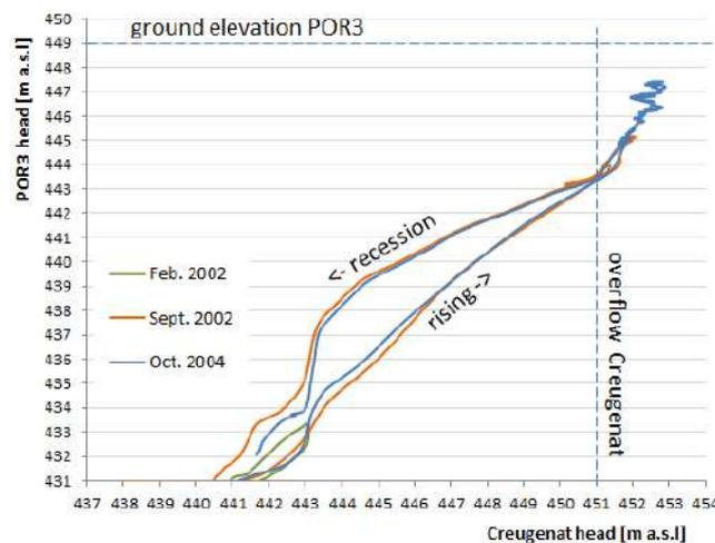
Figure 6—4. Hydraulic relationship between groundwater heads in POR3 and in Creugenat (for 3 selected flood events in 2002 and 2004); for a strong overflow event of Creugenat the water table in POR3 reaches a maximum at 447.5 m. The plateau at 443 m is clearly visible during the recession.
