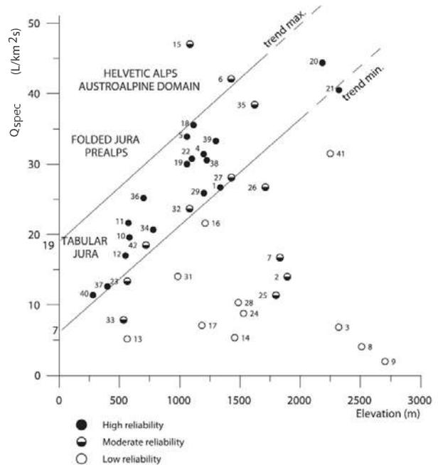
Figure 6. Specific discharge rates  $Q_{spec}$  of the selected systems as a function of elevation (from Figure 5), normalized using the previously established regional deviation grid related to precipitation distribution
