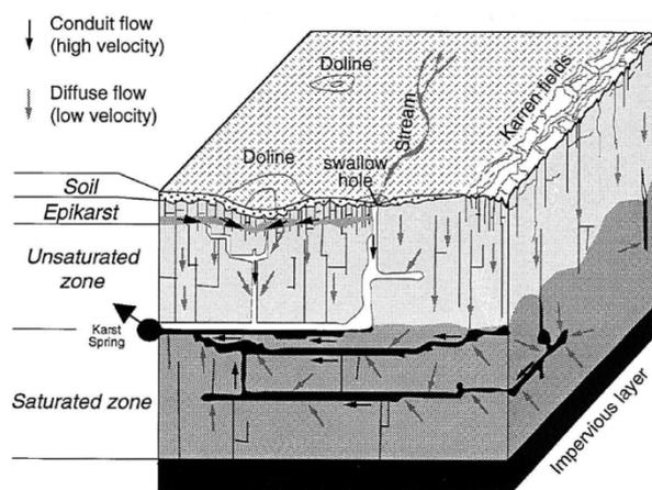
*Figure 2—2. Schematic vertical structuration of epigenic karst aquifers (from Doerfliger [1997]). From top to bottom, karst aquifers are sub-divided into four main zones: Soil, Epikarst, Unsaturated zone and the saturated (phreatic zone). The unsaturated zone may be divided in two zones: the vadose which never floods and the epiphreatic zone which periodically floods*
