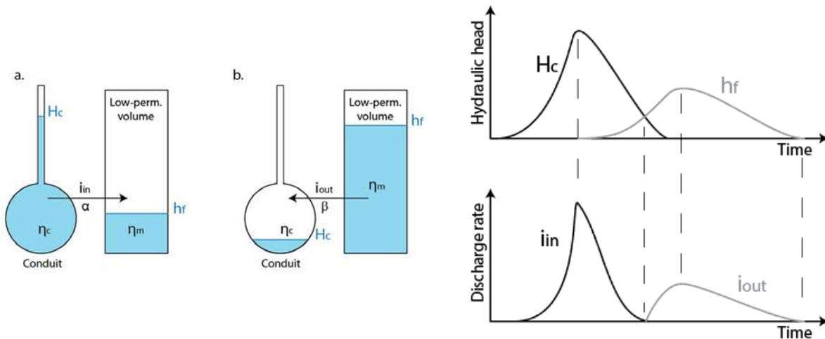
Figure 6—21. Principles of the exchanger functioning for a theoretical flood event;  $i_{in}$  refers to the part of water which is stored in the low permeability volumes while  $i_{out}$  refers to the water released by the low permeability volumes toward the conduits.
