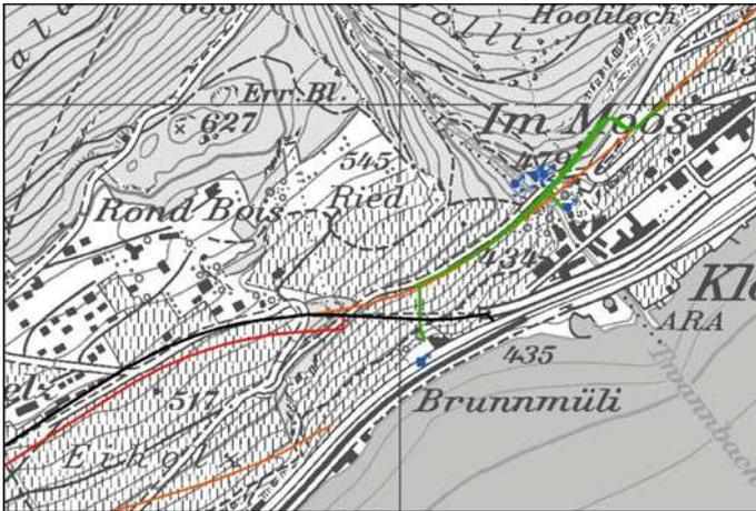
Fig. 1 Site location *Black line* existing main tunnels; *Green line* existing exploration tunnel; *Red line* security gallery (project), *Orange lines* future railway and road tunnels. The Brunnmühle spring (*blue*) emerges at 433 m a.s.l close to Lake Biel. Other springs are visible in the Twannbach canyon (Im Moos)
