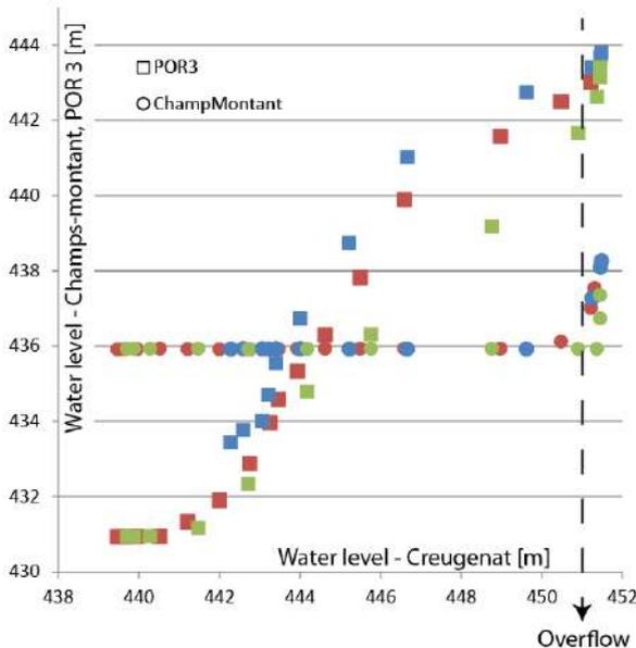
Figure 6—6. Observations from June to July 2012 (i.e. for three flood events of moderate intensity); the water level in the POR3 borehole started to rise simultaneously to the Creugenat flooding while the water table in PdCM does not start rising before the Creugenat overflows.
