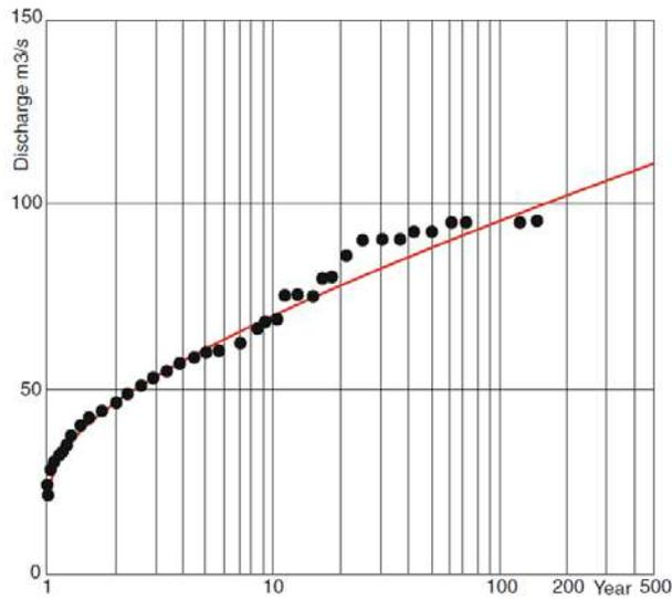
Fig. 35.2 Peak discharge frequency curve of the Suze River in Bienne (Naef and Frauchiger 2009). For  $T$  larger than 10 years peak discharge drops from 68 to 75  $\text{m}^3/\text{s}$  and flattens by about 85 to 95  $\text{m}^3/\text{s}$  for  $T$  between 30 and 150 years
