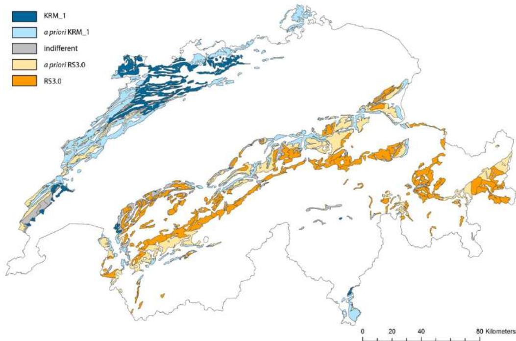
Figure 6—42. Recommended recharge simulation models for karst aquifers in Switzerland. For grey zones, there is no recommended model, RS3.0 or KRM\_1 may be a priori used providing the same interval of confidence; on the blue zones, KRM\_1 could be applied with a high degree of confidence (dark blue) or a moderate degree of reliability (light blue); on the orange zones, RS3.0 should be applied with a high degree of confidence (dark orange) or a moderate degree of reliability (light orange).
