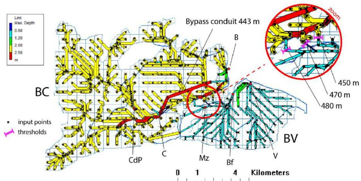
*Figure 6—30. The BC/BV complete SWMM model; colors refer to the diameter of the conduits (Link Max. depth). The model entails the three additional thresholds between the two systems at 450, 470 and 480 m a.s.l., and the long and large by-pass conduit at 443 m in the downstream part of the BC karst system (3 m of diameter).*
