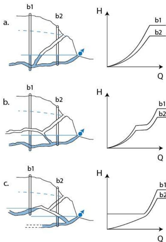
Figure 6—44. Hydraulic functioning for high-flow conditions for three types of situations: **a.** Simple functioning, **b.** By-pass functioning, **c.** Threshold functioning. The network type may thus be inferred from the relationship between hydraulic head ( $H$ ) and discharge rate ( $Q$ ). Such relations provide indications on the conduit organization and on the existence of several conduit levels.
