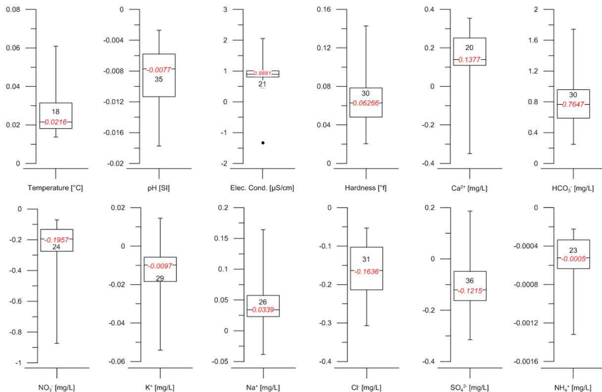
Figure 10—4. Whisker-Box plots showing the evolution of groundwater compounds in Jurassic karst aquifers for the first dataset (Jeannin et al. [Submitted]); the upper graphics refer to parameters related to carbonate dissolution while the lower graphics refer to other parameters showing a meaningful trend. For each parameter, plain values refer to the numbers of stations where the trend
