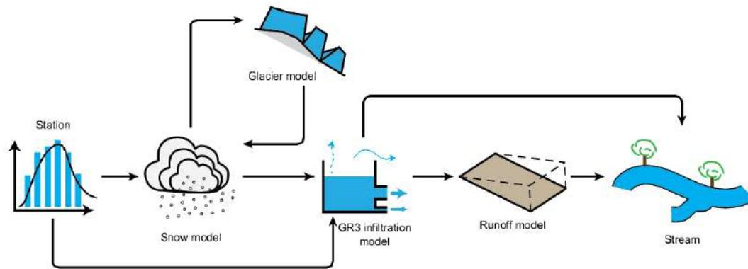
Figure 6—15. Routing principles of the RS semi-distributed software: details of a sub-catchment (i.e. for a given elevation range, here 200 m). Measured or inferred meteorological parameters ( $P$ ,  $PET$ ) are transferred to the GR3' reservoir which provides a part of surface runoff (SWMM module) and a part of infiltration
