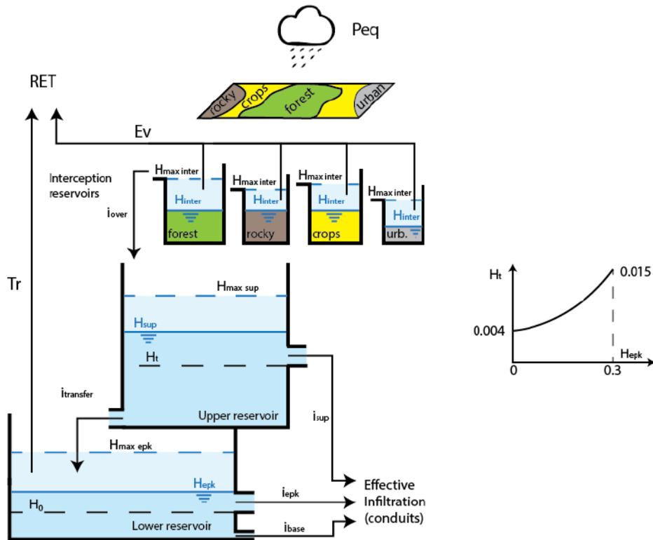
Figure 6—18. Reservoirs organization in KRM\_1; the model entails three cascading reservoirs: the Interception reservoir and the Upper and Lower reservoirs reflecting the tandem soil / epikarst.  $P_{eq}$  is computed with RS3.0. Resulting time series are the effective infiltration (i.e. the water penetrating the conduits).
