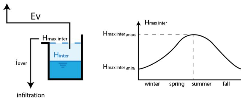
Figure 2—9. Structuration of interception reservoir;  $H_{max\ inter}$  fixes the storage capacity which evolves with the seasons,  $H_{inter}$  is the stored water,  $Ev$  the losses by evaporation and  $i_{over}$  the part of water infiltrating through the soils.
