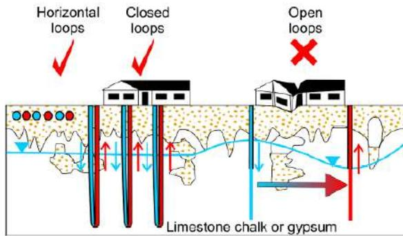
Figure 3—5. Open-loop systems in karst aquifer enhance sediments mobilization or dissolution and may provoke land-subsidence (Cooper et al. [2011]). These mechanisms frequently occur in confined /semi-confined aquifers. This lead UK authorities to develop a decision support tool (GeoSure) which gives indication on areas to karst collapses susceptibility and recommends the type of devices to implant (open or close loop).
