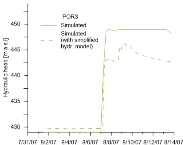
Figure 6—36. Simulated variations of the water table in POR3 for the flood-event of August 2007 [no existing measurements]; simulation results obtained with the simplified hydraulic model (see Appendix 10.14) are plotted for comparison.
