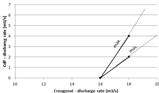
Figure 6—8. Supposed hydraulic relationships between the Creugenat discharge rate and the CdP discharge rate according to a min. and to a max. hypothesis.
