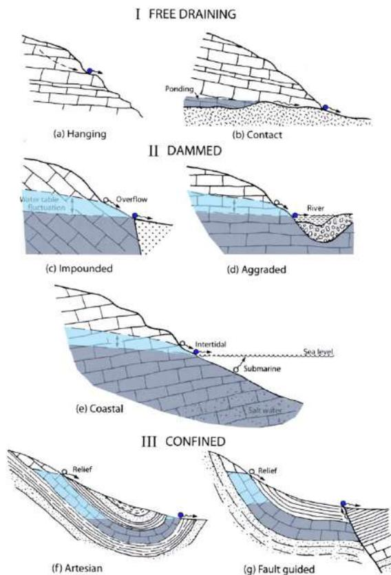
*Figure 2—7. Karst springs are mainly of three types depending on the context of emergence: free draining springs, dammed springs and confined springs (figure from Ford and Williams [2007]). Whatever the context, if the epiphreatic zone shows significant fluctuations, one or several overflow spring(s) may exist upstream from the permanent one(s).*
