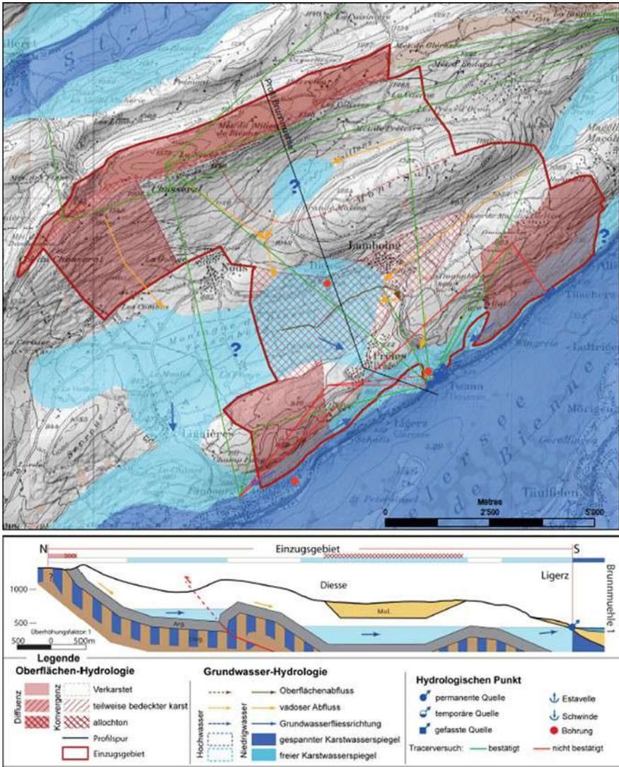
Fig. 4 Preliminary catchment area of the Brunnmühle karst system; the area is 66 km<sup>2</sup> wide but presents divergent parts with the adjacent karst systems
