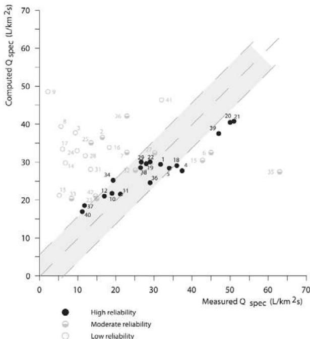
Figure 7. Computed specific discharge rates  $Q_{spec}$  for the 42 flow systems using the mean trend function (after regionalization) of their respective measured  $Q_{spec}$ . The 1 : 1 ratio line represents a perfect match between measured and computed values using the mean trend while the grey band represents the confidence interval between minimum and maximum trends
