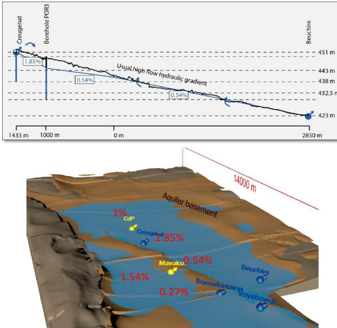
Figure 6—14. The shape of the hydraulic gradient for usual high-flow conditions can be sketched for BC and BV systems. CdP and Mz are still inactive for these conditions.
