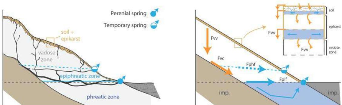
Figure 2—5. Schematic cross-section of a karst flow-system (alpine or jurassian environment); imp.: aquifer basement, **Fvv**: vertical vadose flows, **Fvc**: basement-controlled vadose flows, **Fplf**: phreatic low-flows, **Fphf**: epiphreatic flows (figure from Malard [2013]).
