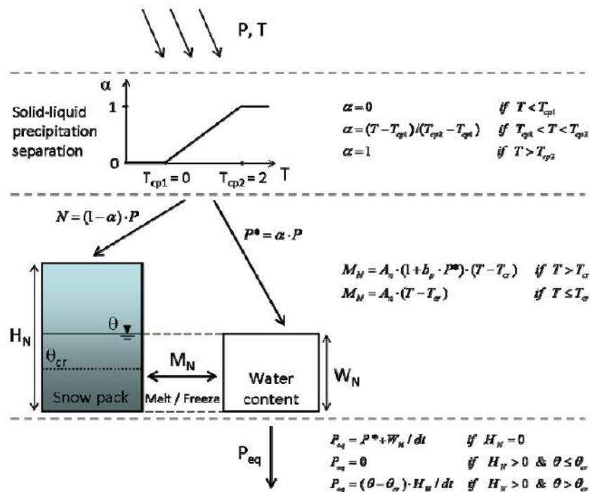
Figure 6—16. Details of the snowpack sub-model of RS3.0. This simulates the evolution of the snow (deposit and melt) as a function of the temperature (T) and precipitation (P) producing an equivalent precipitation (P<sub>eq</sub>) used as input for the glacier or for the GR3 infiltration sub-model (fig. from e-dric [2012])
