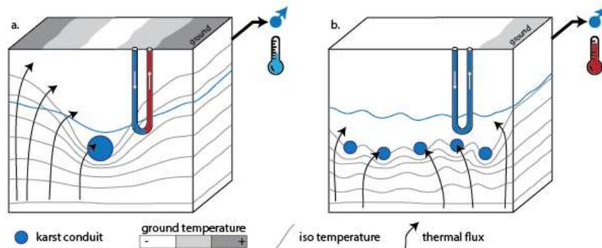
*Figure 3—4. Considering that conduits are efficient for heat drainage, their density and distribution within the massif and the groundwater flux impact the ascending geothermal heat flux. At some locations, aquifers of type (a.) reveal favorable for the implantation of geothermal probes while karst systems of type (b.) may offer more interesting conditions for springs heat exploitation as most of the geothermal flux is absorbed by the flows and carried out at the spring.*
