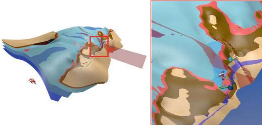
Fig. 3 Perspective view of the geological 3D model of the site (8km along the east-western axis and 6km along the north-southern axis); the tunnel (green pipe) develops along the bedding planes below the Purbeckian marls (red layer)
