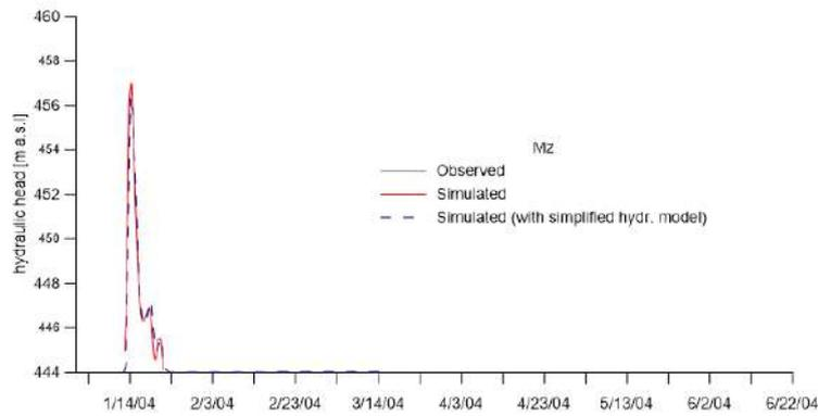
Figure 6—32. Calibration results of the hydraulic heads variations for the borehole POR3 and the Mavaloz cave (Mz) over a selected period (Jan. to Jun. 2004) are compared with the measurements (only for POR3, daily mean values) and the results of the calibration performed with the simplified hydraulic model (see Appendix 10.14)
