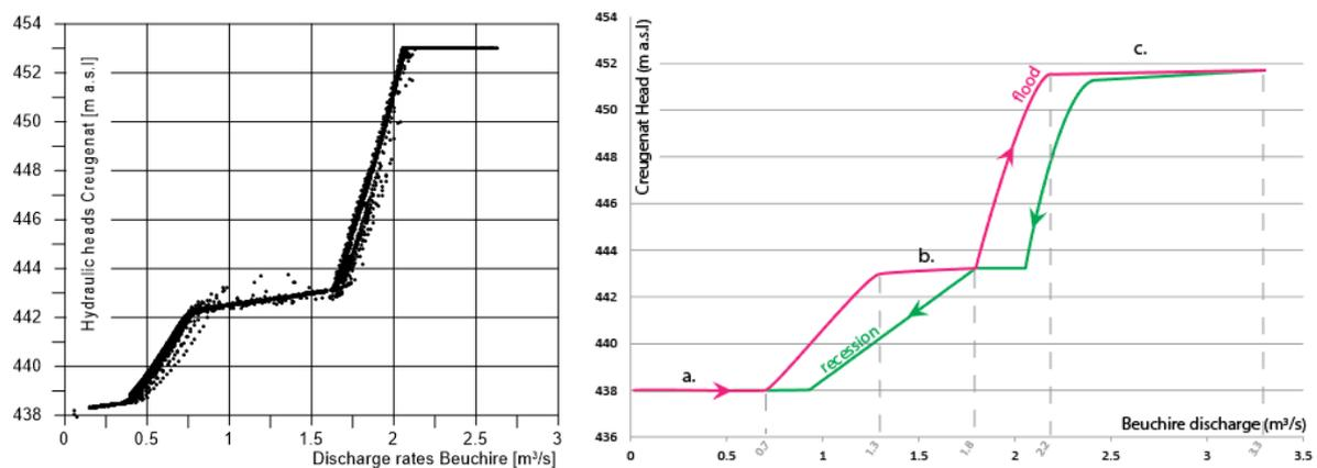
Figure 10—14. Hydraulic relationship between the discharge rate at the Beuchire spring and the evolution of the hydraulic head in the Creugenat (left: simulated, right: observed)
