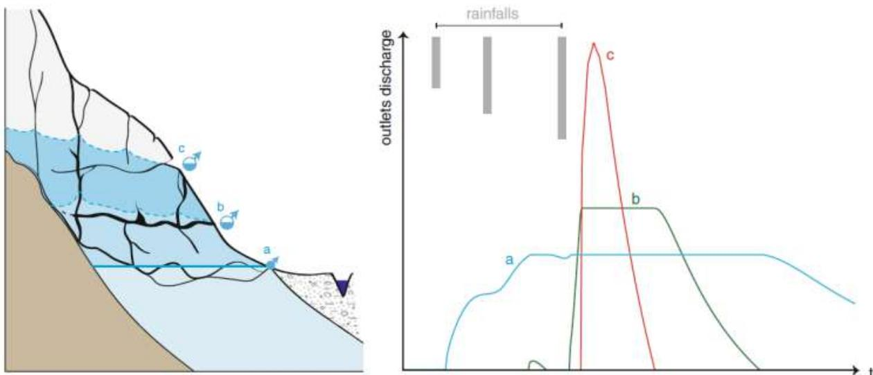
Fig. 35.3 Conceptual model of floods evolution in karst aquifers. While the hydraulic gradient rises in the epiphreatic zone, one part of the coming water is released downstream by overflow springs, and the other part is stored and released later. The position, elevation, discharge capacity and volume of the epiphreatic conduits are the main controlling factors. Depending on the geometry of the aquifer and the rise
